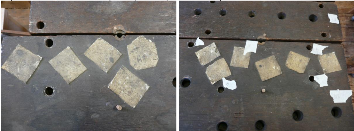
Helper toe-holes covered with leather patches (note the repaired screw holes)
