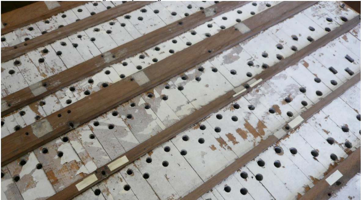
Glueing back the sections of filling-in with hot glue
