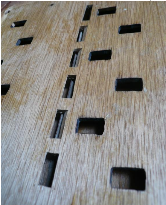
Unused non-return valves between Dulciana and Diapason holes
