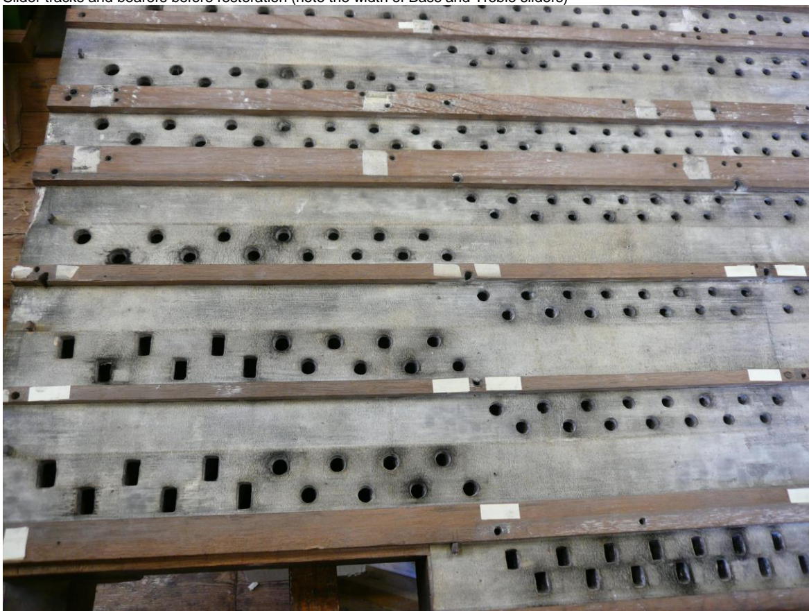
Slider tracks and bearers before restoration (note the width of Bass and Treble sliders)
