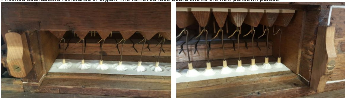
Finished soundboard reinstalled in organ. The removed face board shows the new pulldown purses
