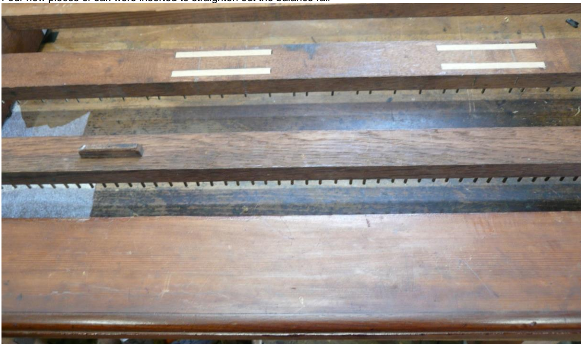
Four new pieces of oak were inserted to straighten out the balance rail
