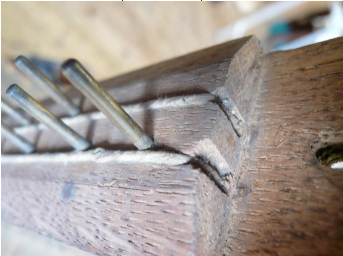
Gut cables anchored in front of the balance-pins with small brads under quite some tension
