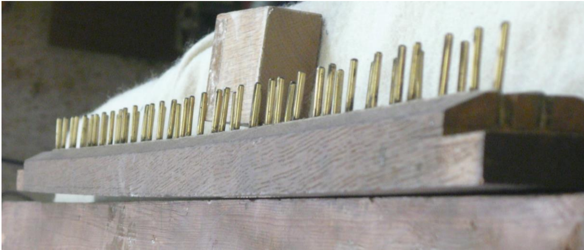
The balance rail shows a severe bend
