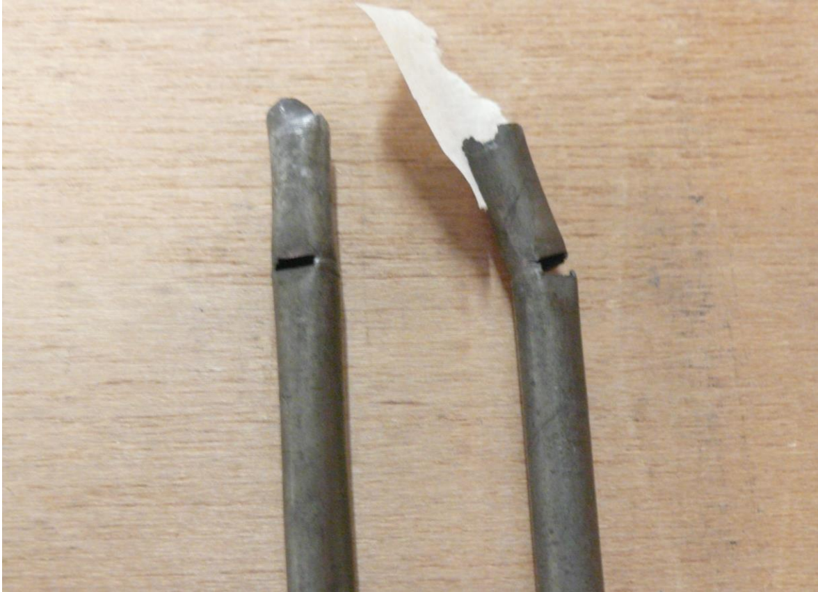
Several pipes in the top of the 17 th rank of the Cornet were in bad condition
