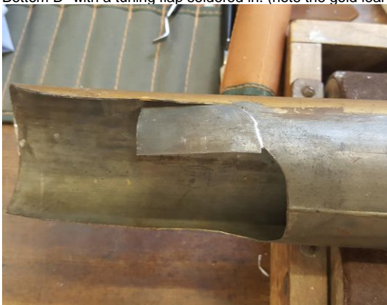
Bottom D# with a tuning flap soldered in. (note the gold leaf on the cut edge)
