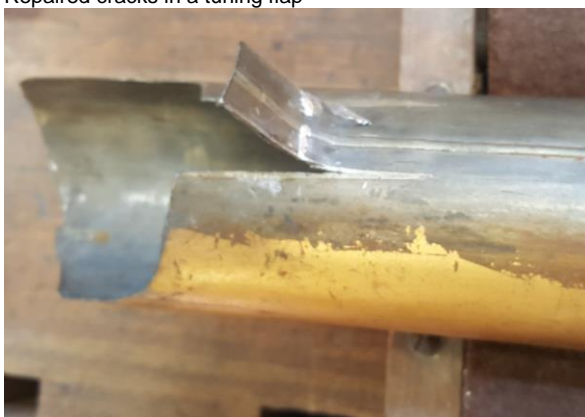
A new tuning flap replacing a missing one
