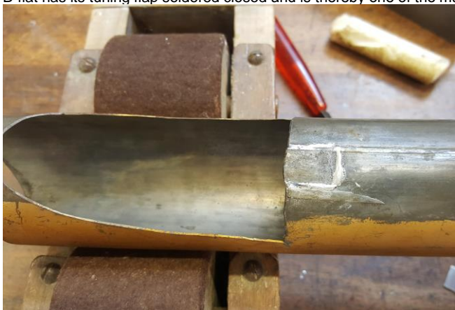
Repaired cracks in a tuning flap
