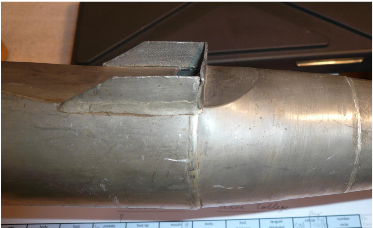
Box beards for the Dulciana (notice the cloth pattern on the inside of the far ear)
