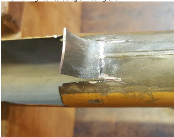
A new tuning flap replacing a missing one
