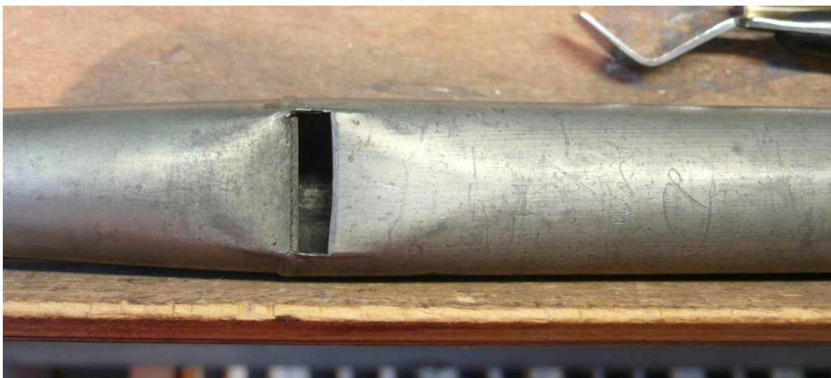
Detail of the scoring of the smaller pipes. (Note the thin languid)
