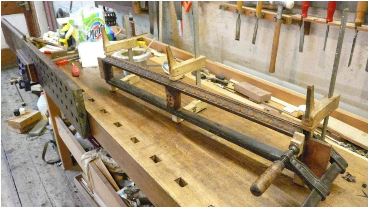
Rail with two letterbox-slots prepared for closing up with a thick veneer
