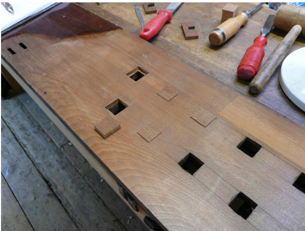
The Bass jamb being restored to the original number of holes
