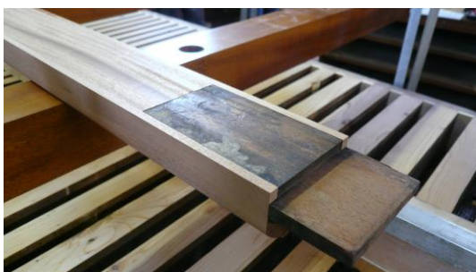
The old tenon inserted into the back of the new case rail
