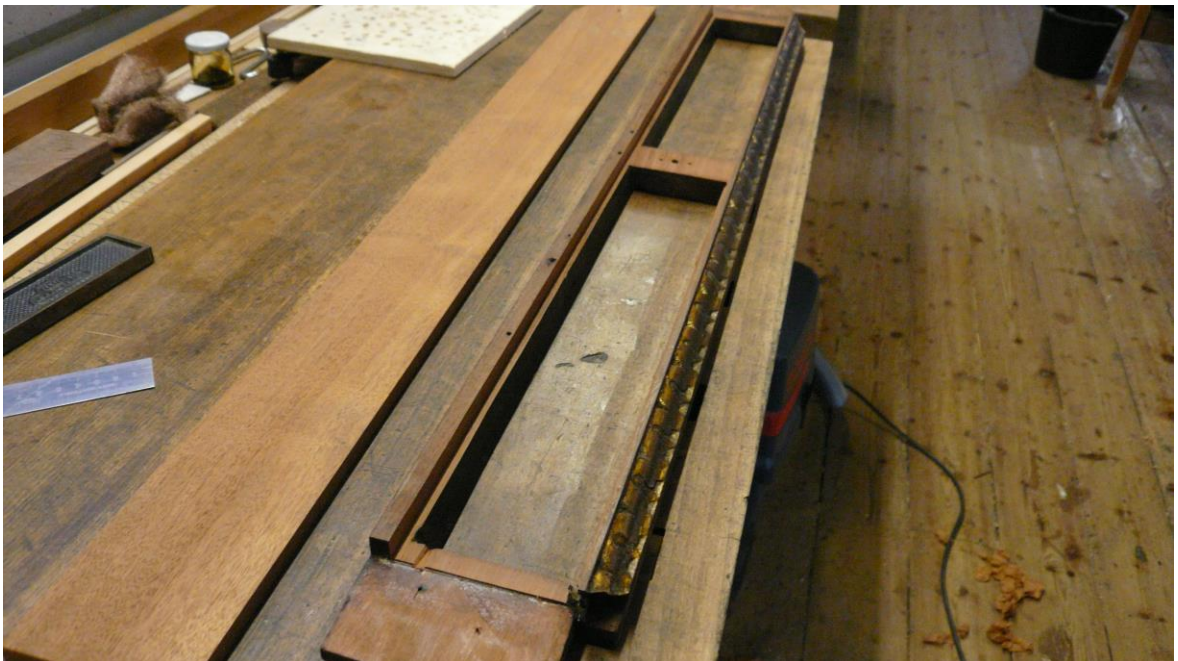
Rail with two letterbox-slots prepared for closing up with a thick veneer
